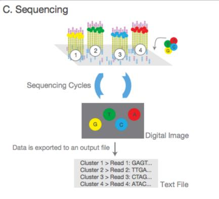
Sequencing reagents, including fluorescently labeled nucleotides, are added and the first base is incorporated. The flow cell is imaged and the emission from each cluster is recorded. The emission wavelength and intensity are used to identify the base. This cycle is repeated "n" times to create a read length of "n" bases.
